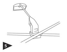
OPTIONAL Attach lights to top of frame by sliding the plastic X Blocks under the frames cross sections.
