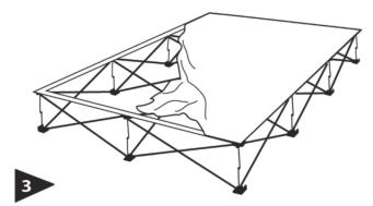
Work in continuous direction around the frame until graphic is completely attached.
