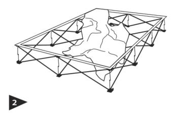
Starting at one corner, attach Velcro® on graphic to Velcro® on frame. Overlap Velcro® of graphic a 1/4" on all sides of Velcro® of frame. Note: Velcro® should not be flush.
