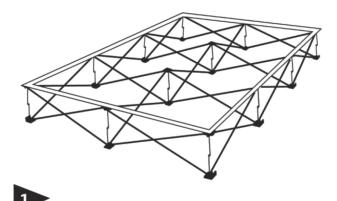
Assemble frame and lay flat on its back. Remove existing graphic.
